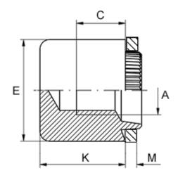
Female thread A = M3,5Height K = 9.0Min thread length C = 4.0Outer diameter E = 10.0Plate thickness = 0.5 to 0.6
